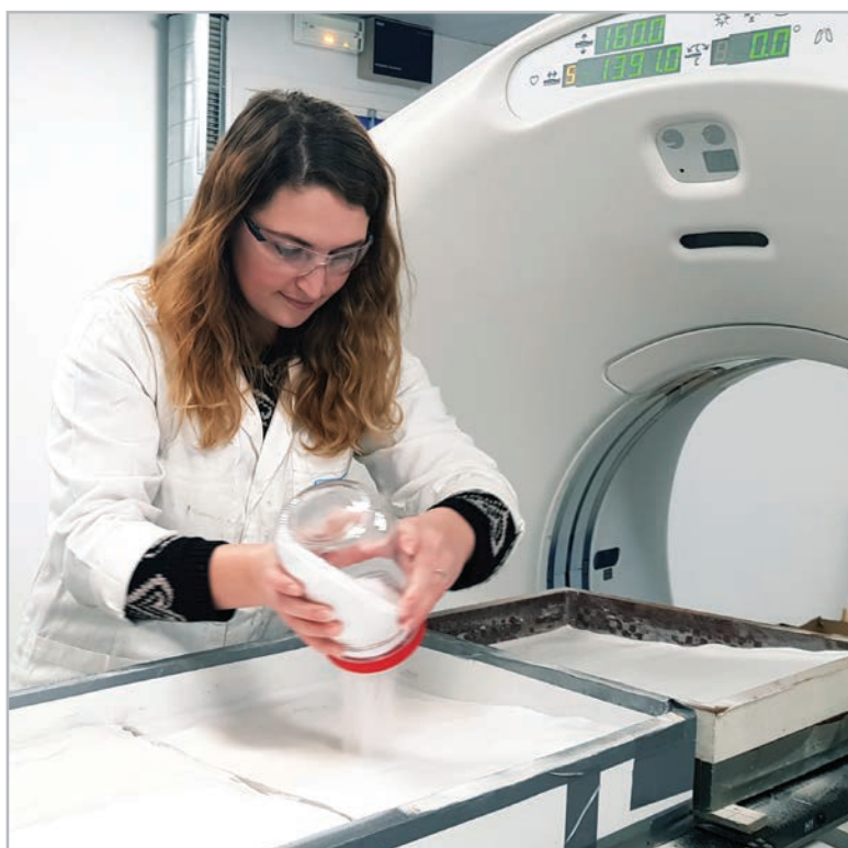
Analogue modelling in action: applying additional sand layers at certain time intervals during model runs (left), and ensuring even distribution of sand layers (right)
